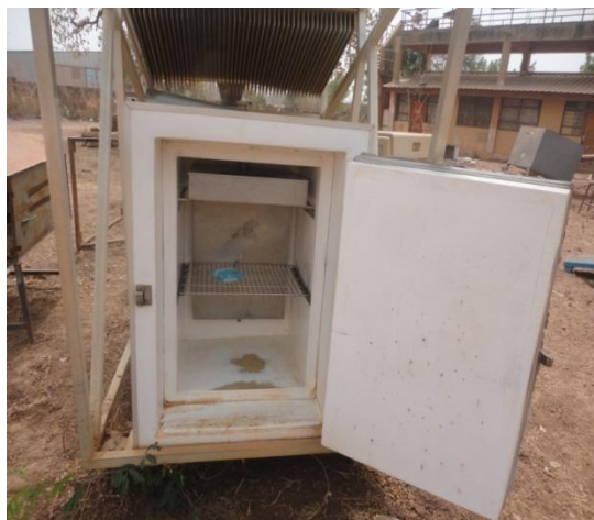
Figure 1 : Photo of the evaporator and the chest
